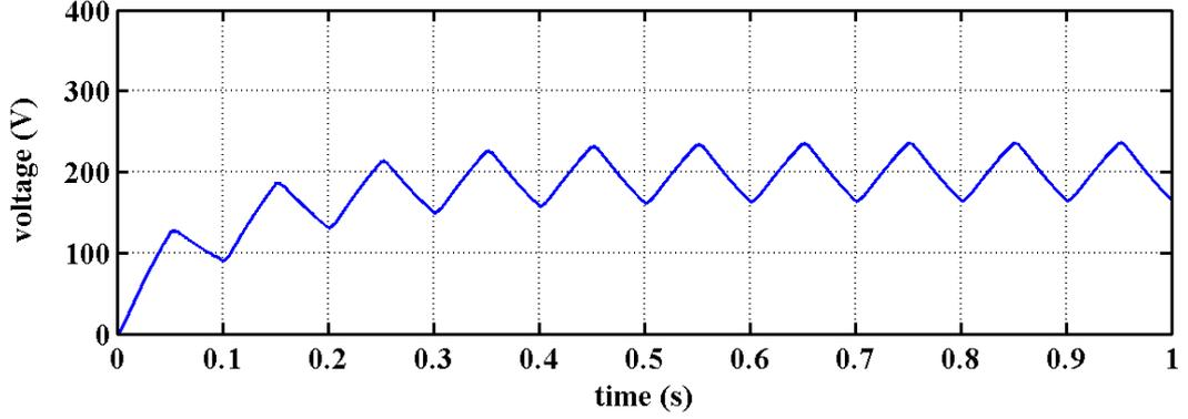
**Figure 2.4.5: Transient build-up of the capacitor voltage**
