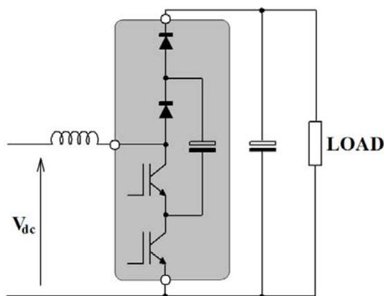
**Figure 2.3.2: Boost regulator using low-side chopper module**
