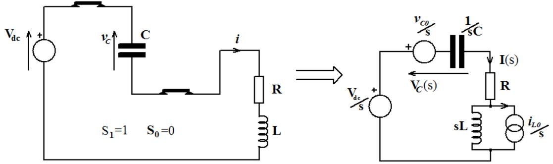
**Figure 2.4.3: Laplace equivalent circuit for switch state 2**
