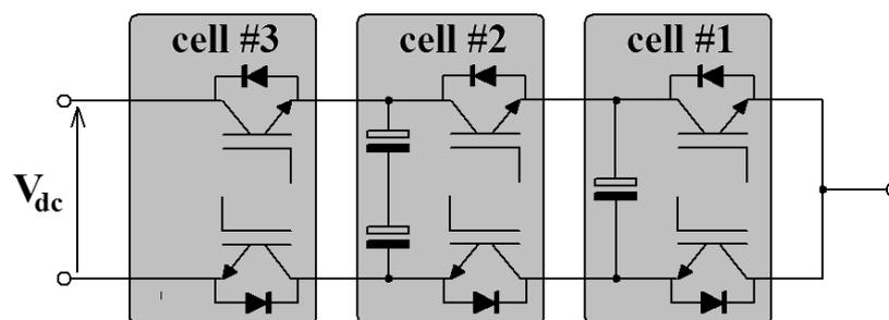
**Figure 2.3.6: Four-level inverter limb**
