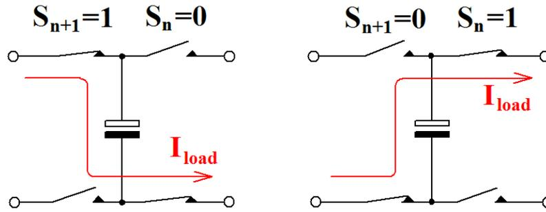
**Figure 2.3.8: Current flow paths in a cell capacitor**
