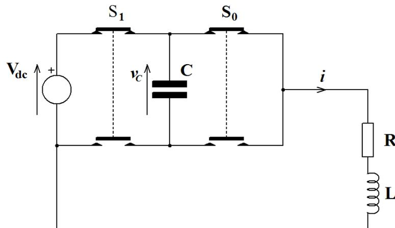
Figure 2.4.1: Two-cell inverter limb
