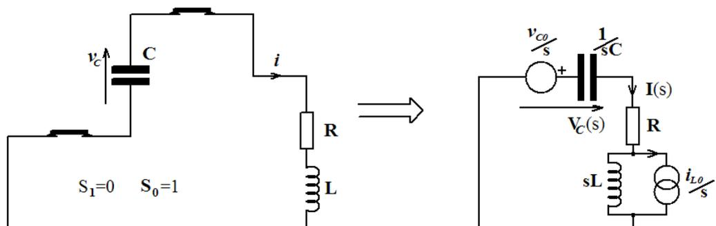
Figure 2.4.2: Laplace equivalent circuit for switch state 1
