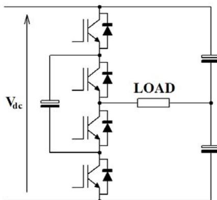
**Figure 2.3.4: Half-bridge circuit**
