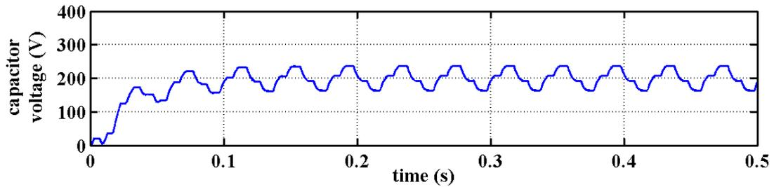
**Figure 2.4.8: Capacitor voltage build-up from inert state**
