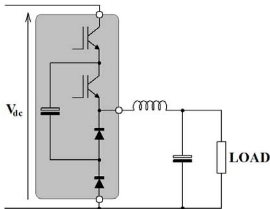
**Figure 2.3.1: Buck regulator using high-side chopper module**
