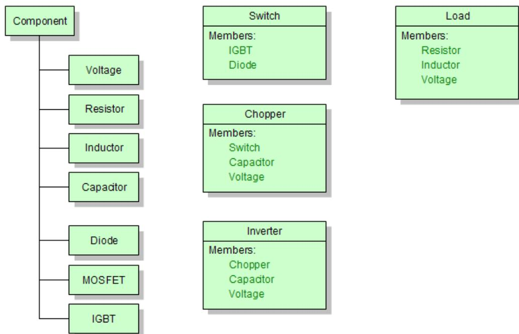
**Figure 2.5.1: Class hierarchy and derived simulation classes**
