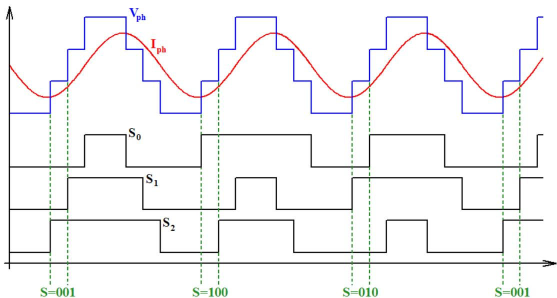
**Figure 2.3.9: Firing waveforms for simple state rotation balancing in a three-cell inverter limb**
