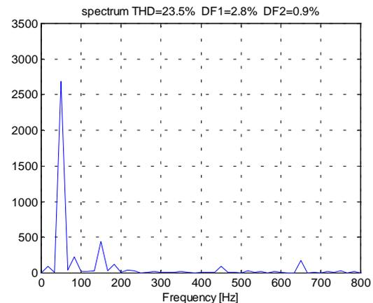
Figure 7: Load Voltage Spectrum - High THD
