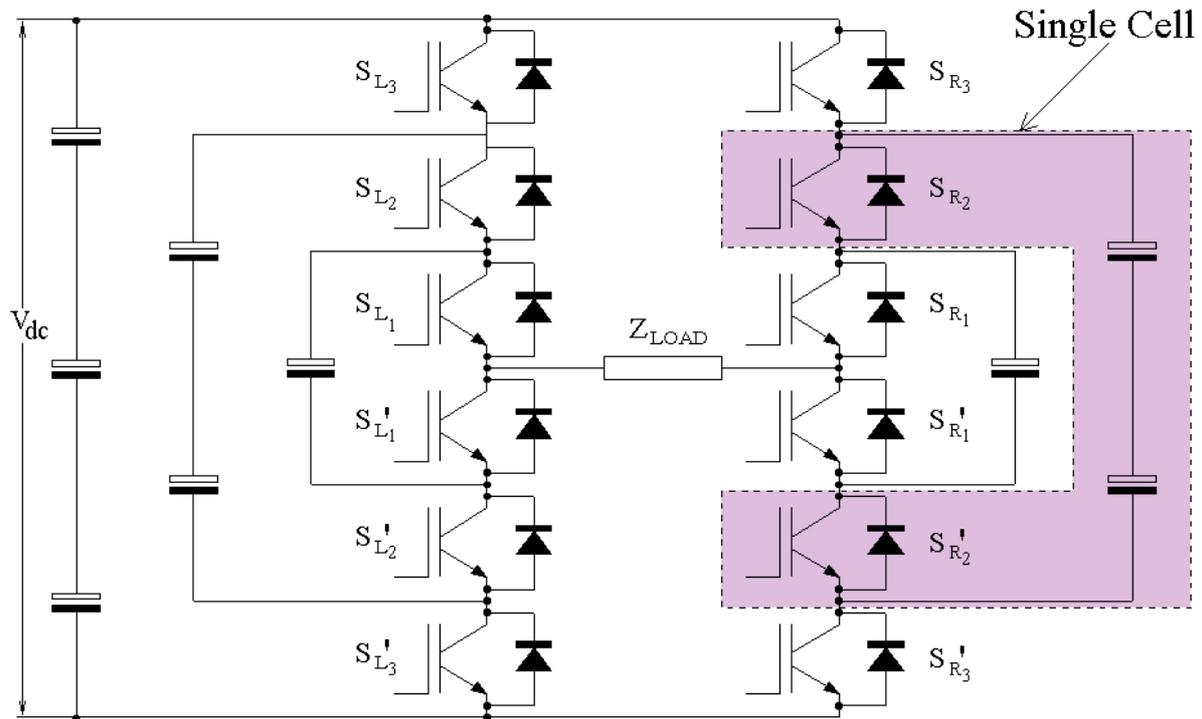
Figure 1: Three-Cell Inverter
