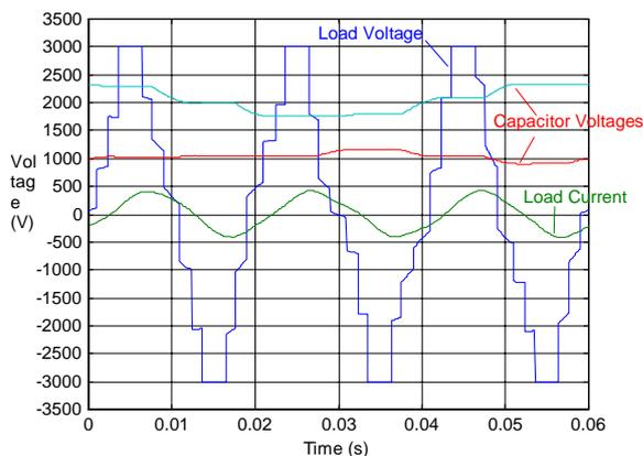
Figure 6: Load Waveforms - High THD
