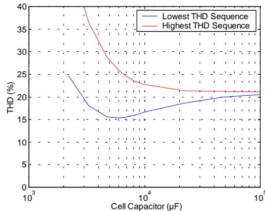
Figure 6: Switching Pattern THD Variation With Cell-Capacitance
