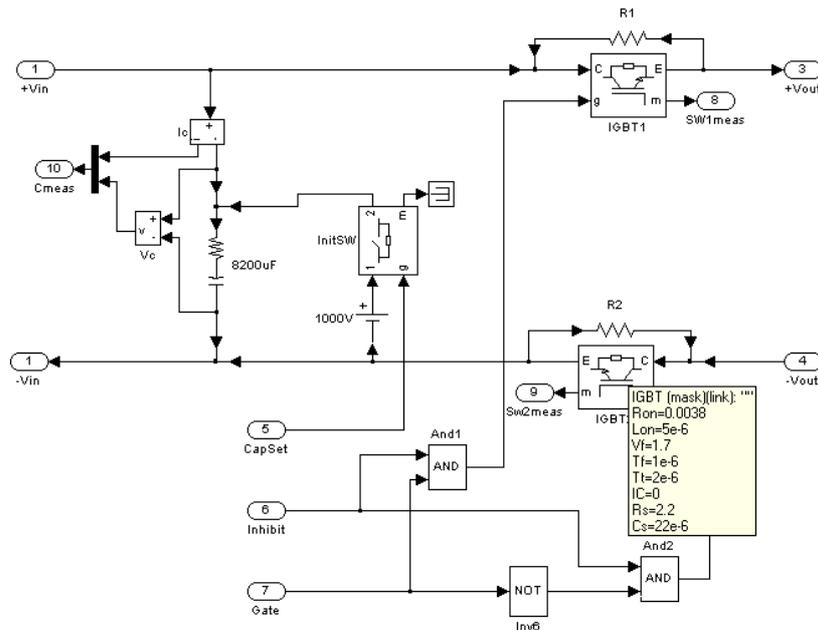
Figure 9: Inverter Cell Simulation Schematic
