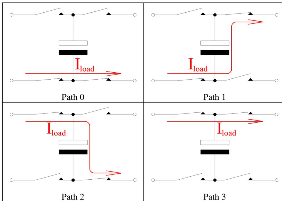
Figure 2: Cell-Capacitor Current Paths
