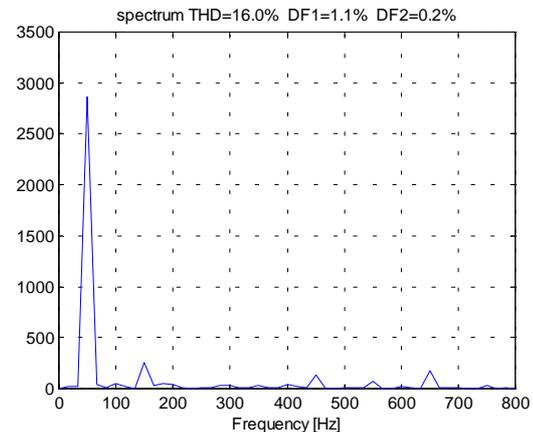
Figure 5: Load Voltage Spectrum - Low THD
