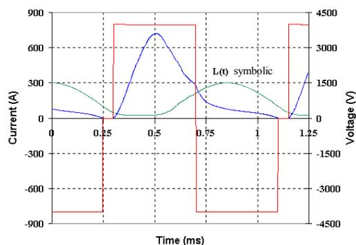
Figure 6: Simulated Waveforms at 17600 rev/min, 1087 Nm
