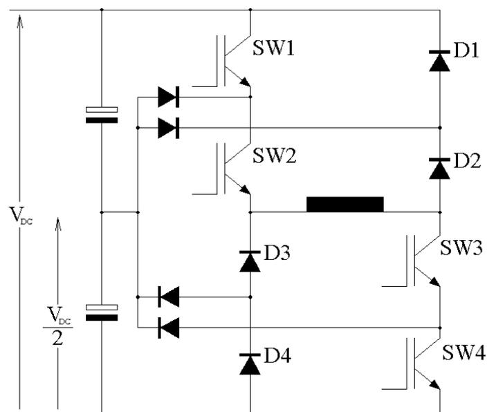
Figure 1: Two-level Diode-Clamped Asymmetric Half-Bridge Phase Limb
