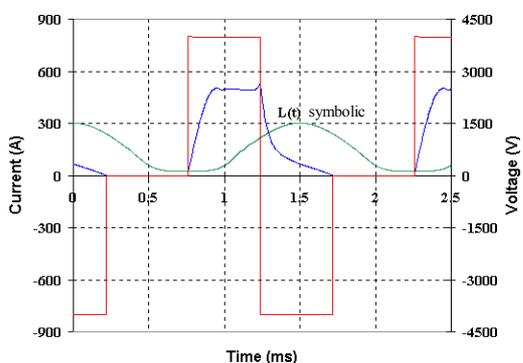
Figure 7: Simulated Waveforms at 10000 rev/min, 1140 Nm
