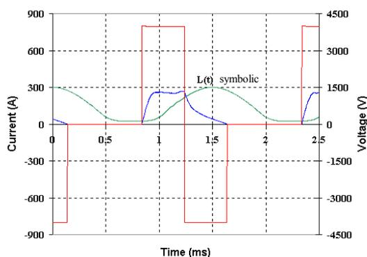
Figure 8: Simulated Waveforms at 10000 rev/min, 540 Nm
