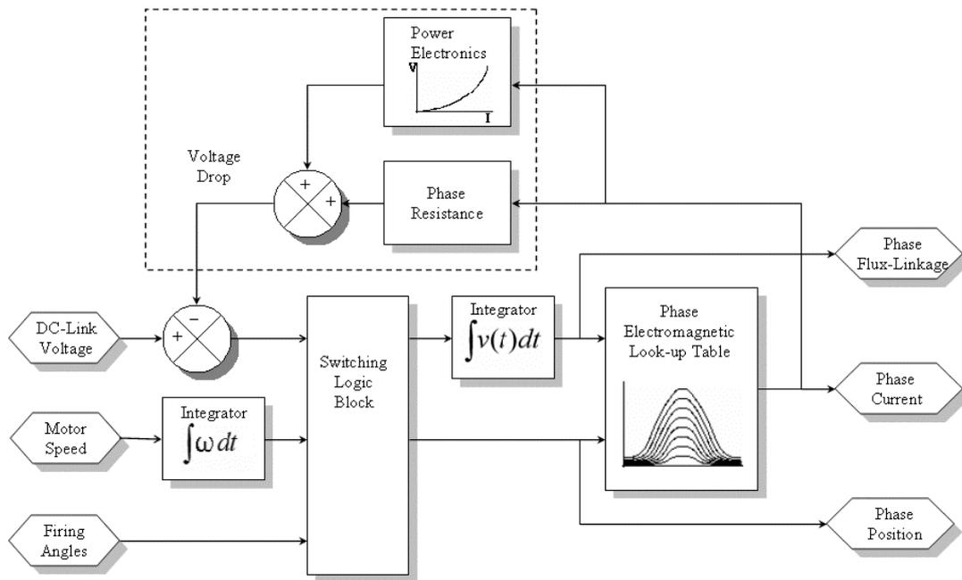
Figure 4: Block Diagram of SR Drive Computer Simulator
