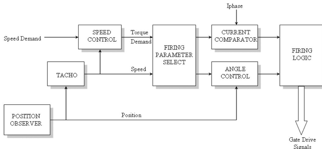
Figure 2: Typical SR Controller Block Diagram
