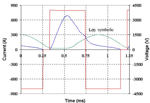
Figure 5: Simulated Waveforms at 16780 rev/min, 1066 Nm
